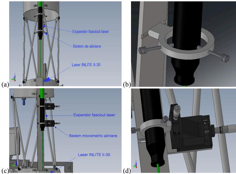
Figure II.e. (a) Overview of the alignment system and (b) detailed view of the “classic” fixation/alignment system for the emission module c) Overview of the alignment system and (d) detailed view of the micrometric fixation/alignment system for the emission module.
