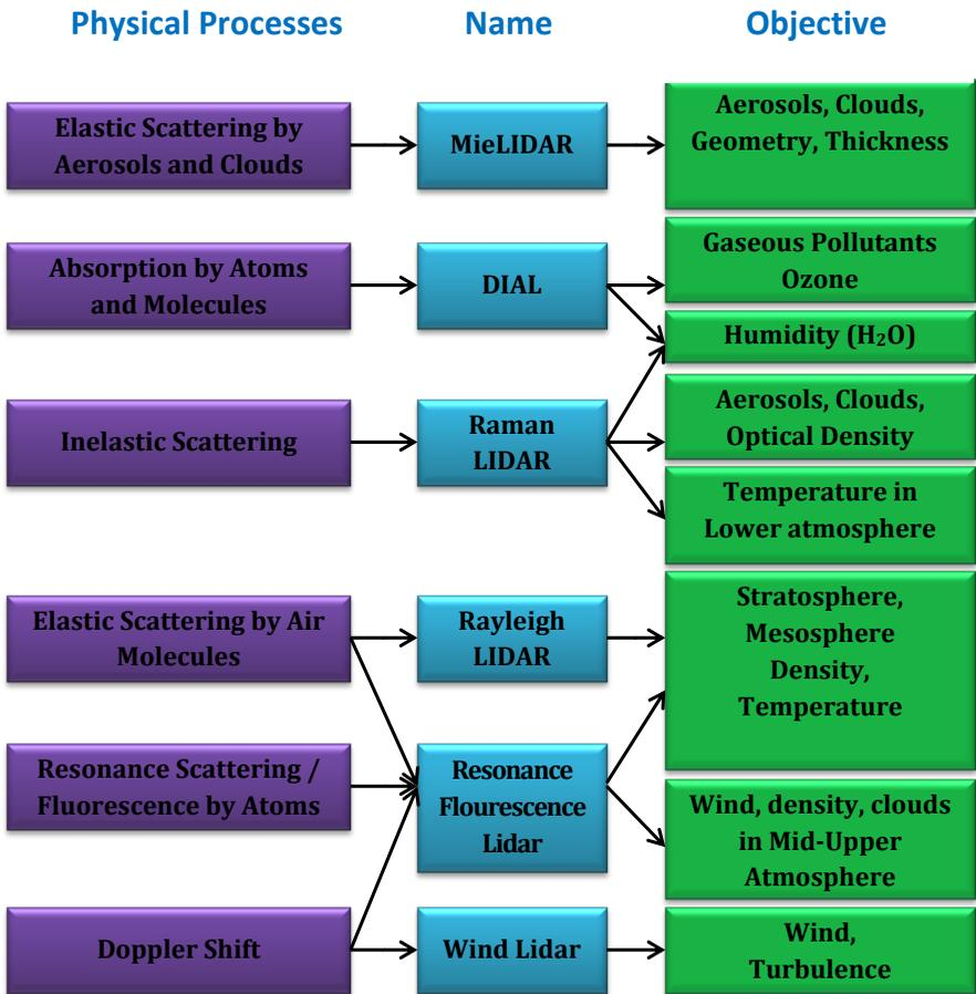
Figure I.3. Types of Lidar systems.
