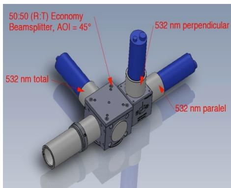
Figure II.7. <sup>ESY</sup>Lidar reception module for depolarization studies
