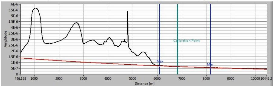
Figure II.13. Rayleigh fitted and optimized Lidar signal.
