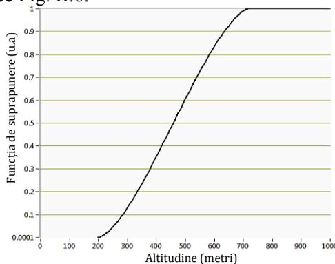
Figura II.6. The overlapping function characteristic to the *ESY*Lidar system.
