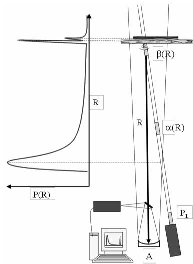
Figure I.2. Operating principle of a Lidar system [13].
